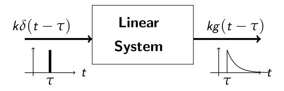
The following sketches the derivation of the convolution integral.
