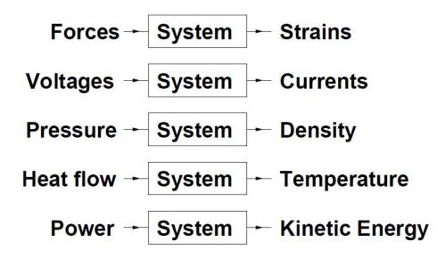
In a linear system the output (y(t)) is computed as some linear combination of the input (x(t)) (including inputs from the past, if we are considering a system with a time-varying input and output).
