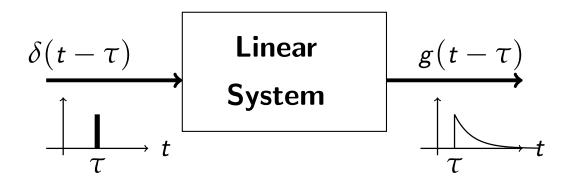
A scaled impulse at time t = 0 produces a scaled impulse response.
