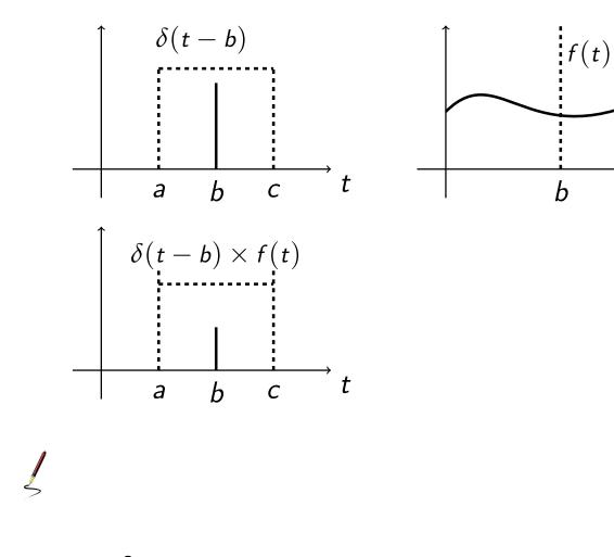
$\int_{a}^{c} \delta(t-b) dt = 1 \text{ provided } a < b \text{ and } c > b$
