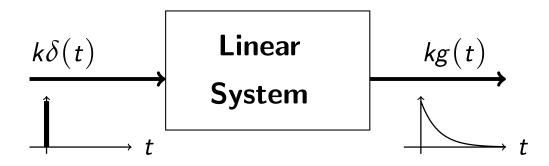
An impulse that has been scaled by k and delayed to time  $t = \tau$  produces an impulse response scaled by k and starting at time  $\tau$ .
