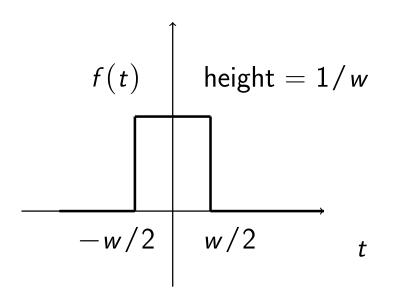
As  $w \to 0$  the pulse f(t) becomes narrower and taller. In the limit as  $w \to 0$  the pulse f(t) becomes a delta function:  $\delta(t)$ .
