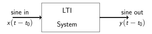
Suppose, for example, that an input of  $sin(\omega t)$  is passed through an LTI system and produces an output of  $sin(\omega t) + sin(2\omega t)$ , ie that the frequency of the input is not preserved in the output:
