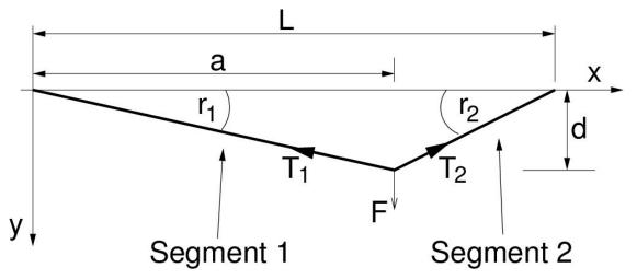
To find g(x, a) we first work out the maximum displacement, d, for a point load, F = 1, at position a.
