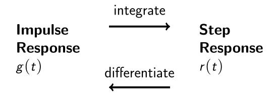
**Example:** Find the output, g(t) of a linear system with step response  $r(t) = 1 - e^{-5t}$  when the input is the delta function  $\delta(t)$ .
