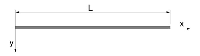
Consider a taut string suspended between two points a distance L apart. It is subject to a uniform loading of K per unit length which results in a *small* displacement.
