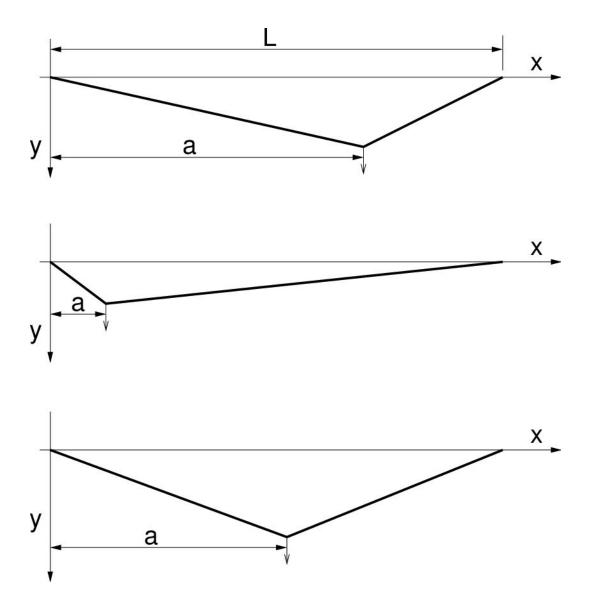
But a normal impulse response is not possible because the shape of g changes depending on the position of the point load along the string. We have a function g(x, a)where the point load is at position a. The function g that gives the displacement under a point load depends on both the position of the load, a, and the position at which you want to know the displacement, x. Linear Systems
