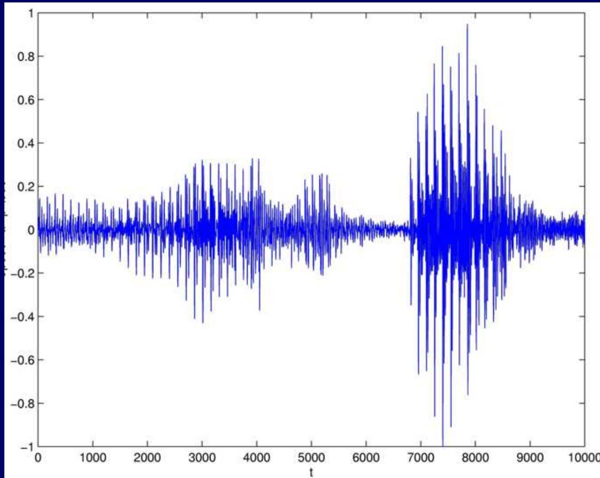
Figure 1: Speech data. 0.62s of a US male speaker saying the words '...rewarded by...'. Sample rate 16kHz, resolution 16-bit, from the TIMIT speech database
