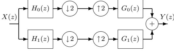
**Fig. 2.** 2-band analysis and reconstruction filter banks.
