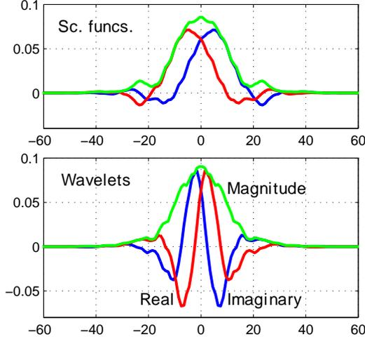
**Fig. 6.** Scaling functions and wavelets at level 4 for  $n = 6$ . Red and blue curves show the real and imaginary parts, and the green curves show the magnitudes of the complex waveforms.
