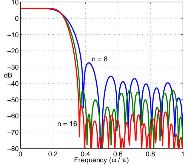
**Fig. 5.** Frequency responses of  $H_{L2}(z)$  for  $n = 8$  (blue),  $n = 12$  (green) and  $n = 16$  (red). Each filter has one predefined zero at  $\omega = \frac{\pi}{2}$  and one at  $\omega = \pi$ .
