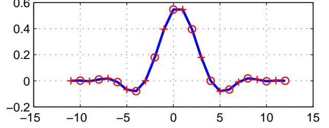
**Fig. 3.** Impulse response of  $H_{L2}(z)$  for  $n = 6$ . The  $H_0$  and  $G_0$  filter taps are shown as circles and crosses respectively.
