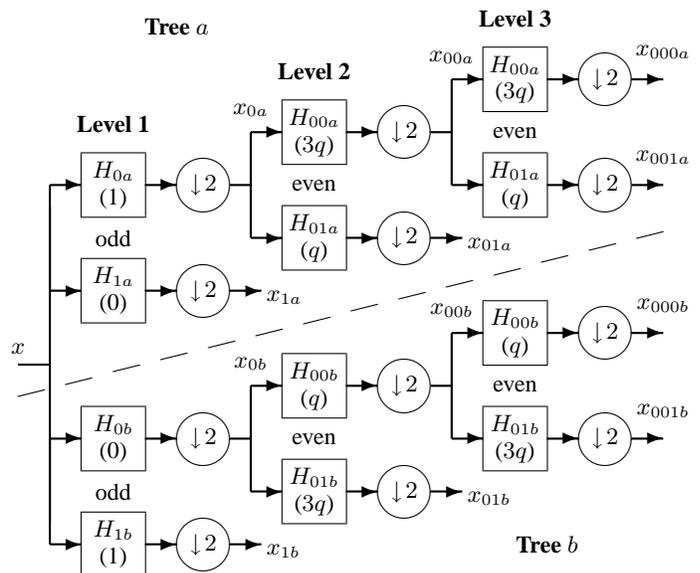
Fig. 1. Dual-Tree Complex Wavelet Transform over 3 levels.
