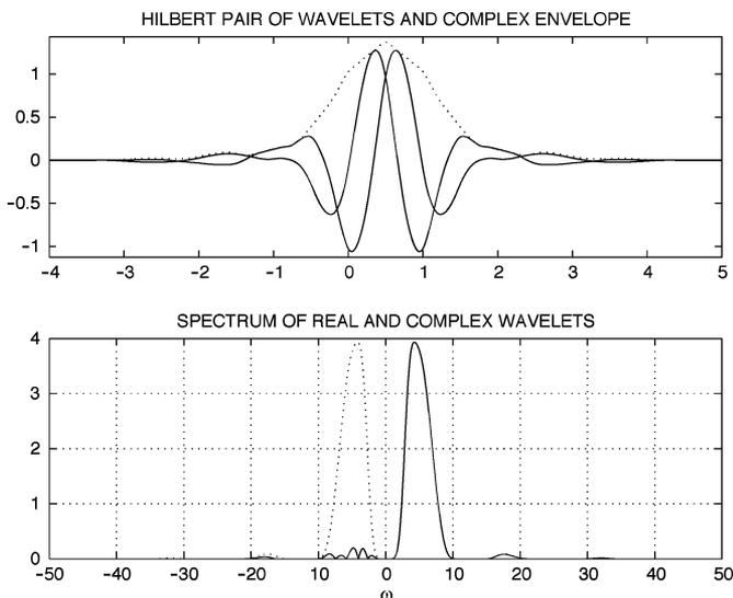
Fig. 3. Orthonormal Hilbert-pair from length 18 CQF using  $a = 0.2407$ . Top diagram: time wavelet functions (solid line) and the magnitude of complex envelope  $|\psi^h(t) + j\psi^g(t)|$  (dotted line). Bottom diagram: spectrum of complex wavelet  $|\Psi^h(\omega) + j\Psi^g(\omega)|$  (solid line) and spectrum of real wavelet  $2|\Psi^h(\omega)|$ .
