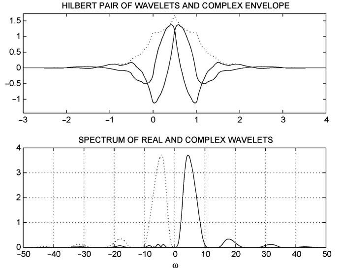
Fig. 1. Orthonormal Hilbert-pair from length 8 CQF using  $a = 0.046$ . Top diagram: time wavelet functions (solid line) and the magnitude of complex envelope  $|\psi^h(t) + j\psi^g(t)|$  (dotted line). Bottom diagram: spectrum of complex wavelet  $|\Psi^h(\omega) + j\Psi^g(\omega)|$  (solid line) and spectrum of real wavelet  $2|\Psi^h(\omega)|$ .
