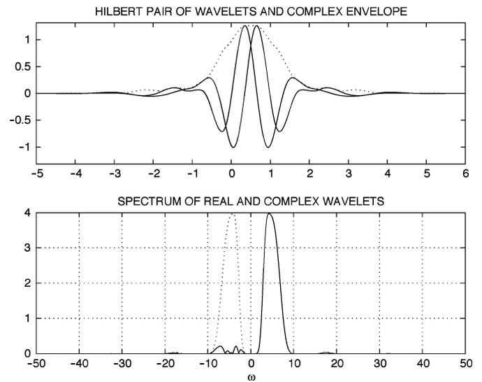
Fig. 4. Orthonormal Hilbert-pair from length 22 CQF using  $a = 0.0240$ . Top diagram: time wavelet functions (solid line) and the magnitude of complex envelope  $|\psi^h(t) + j\psi^g(t)|$  (dotted line). Bottom diagram: spectrum of complex wavelet  $|\Psi^h(\omega) + j\Psi^g(\omega)|$  (solid line) and spectrum of real wavelet  $2|\Psi^h(\omega)|$ .
