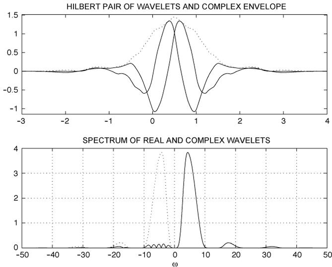
Fig. 2. Orthonormal Hilbert-pair from length 12 CQF using  $a = 0.1824$ . Top diagram: time wavelet functions (solid line) and the magnitude of complex envelope  $|\psi^h(t) + j\psi^g(t)|$  (dotted line). Bottom diagram: spectrum of complex wavelet  $|\Psi^h(\omega) + j\Psi^g(\omega)|$  (solid line) and spectrum of real wavelet  $2|\Psi^h(\omega)|$ .
