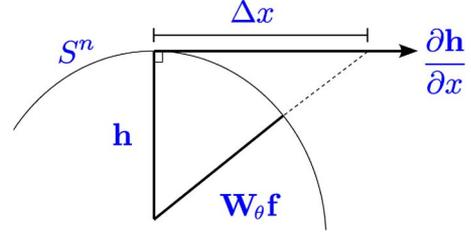
Fig. 6. Shift tolerance problem, simplified in 2-D space. Find the shift distance  $\Delta \mathbf{x}$  along the surface of the hypersphere  $S^n$ , such that the unit vector  $\mathbf{h}$  is rotated into  $\mathbf{W}_\theta \mathbf{f}$ .
