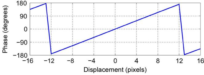
Fig. 5. Step edge orientated at  $15^\circ$  to the horizontal, and placed in the center of a  $128 \times 128$  subimage is decomposed by the DTWCT. The phase angle of the center DTCWT coefficient from subband 1 at the fourth finest scale level is plotted with respect to vertical displacement. Note how the phase completes approximately  $3/4$  of a cycle over the sampling period of  $2^4 = 16$  pixels.
