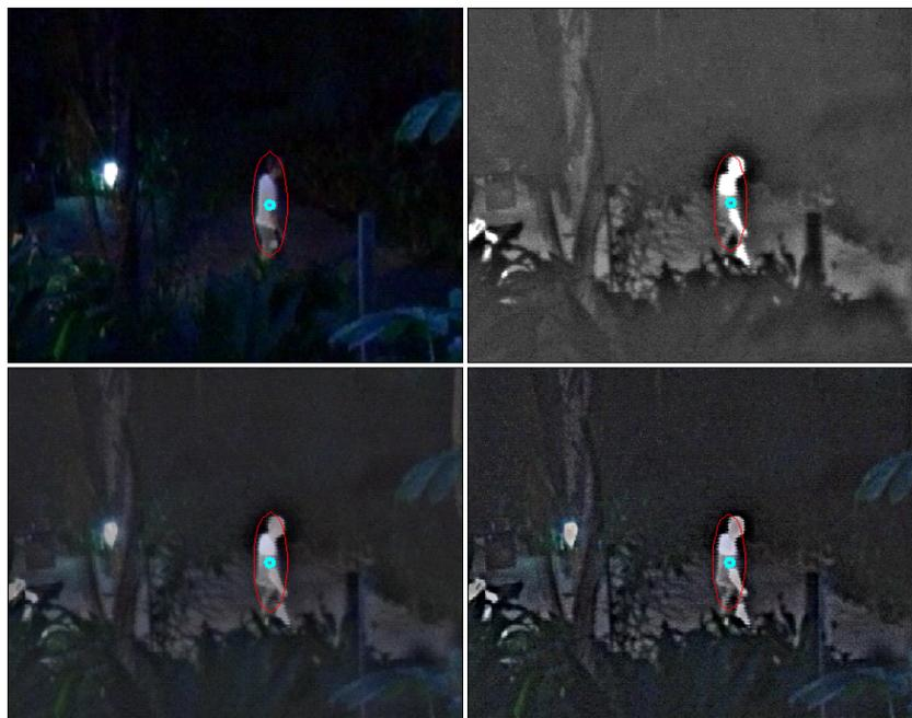
Figure 6: Tracking in an Eden sequence. Clockwise from top left the results correspond to: visible, infrared; DT-CWT fused and average fusion
