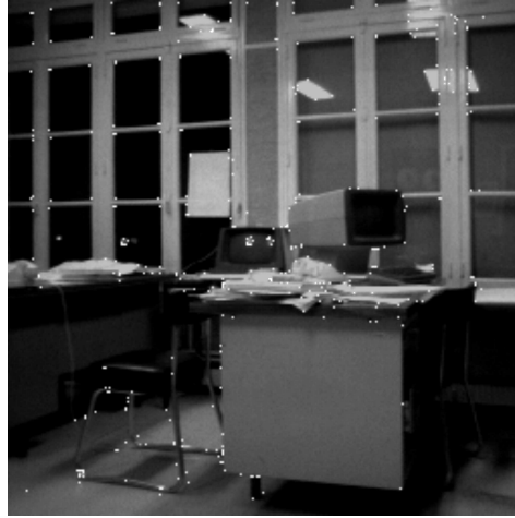
Figure 17: Extraction of corners from an indoor scene
